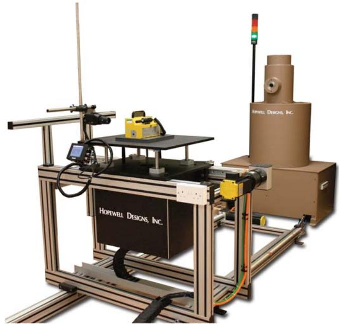
Model GC60 Gamma Beam Irradiator
