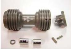
The sources are installed into an aluminum holder called a rabbit. These rabbits are loaded into the irradiator into a rotating carousel. The carousel rotates to align the selected source with the transport tube. The source is moved from the storage position to the expose position by compressed air and held in place by a suction cup. Position of the rabbit is closely monitored with photo eye sensors and vacuum sensors to ensure the source is in the desired location.
